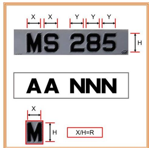
Example: plate geometry and basic syntax
